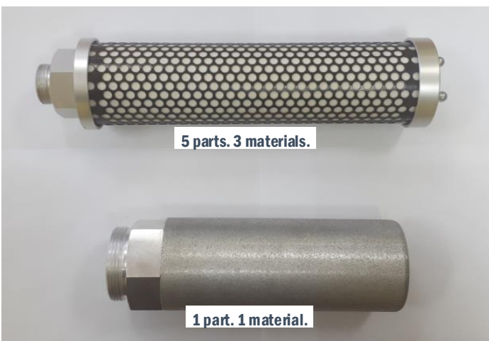
Series application: Compressed air silencers made of open-pore cast aluminum (below) are lighter, smaller, better, cheaper and more sustainable than conventional silencers made of different materials.
