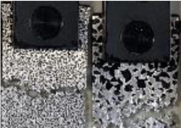
Testing the bond strength of the composite with infiltrated PA6GF30 polymer into large and small pores (injection moulding process).
