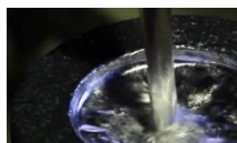
2. Mold filling with Al melt.
