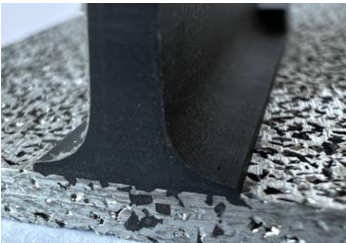
Local functionalization with PA6GF30 polymer in the injection moulding process.
