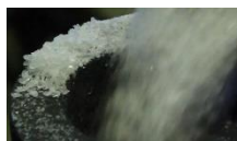
1. Mold filling with salt (NaCl) granules.
