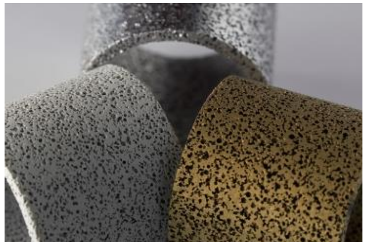
Bushing made of open-cell AISi7 cast aluminum (top) with METAKER® Composites surface (left) and PVD coating (right).
